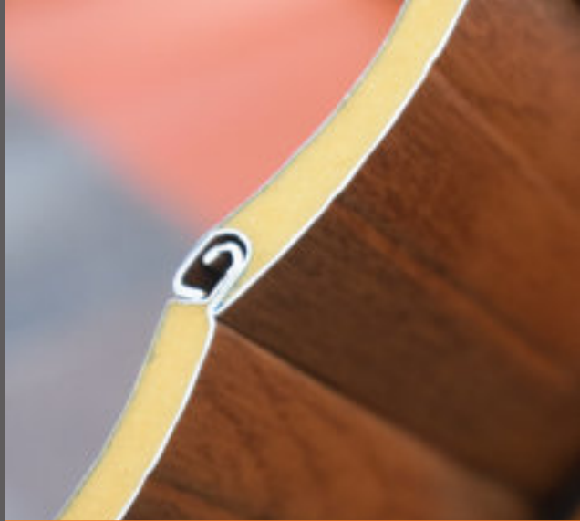
Double skinned aluminium enclosure with a polyurethane foam core
